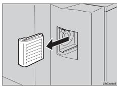
**2** Remove the ozone filter from inside the ventilator hole cover.
